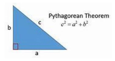
Lets say we have two vectors at right angles. We can draw on the resultant vector and use pythagoras to work out the magnitude (size) of the resultant force. Here are two forces acting on an object at right angles. We can draw on the resultant and this makes a right angled triangle.
