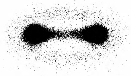
Fig. 8. Charge cloud for \text{H}_2^+
